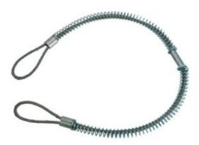
If a hose fails at the fitting area, Raah Safety - Cable Restraints are designed to give limited protection from hose whipping. The Cable Restraint will work on hoses ranging in size from 1/2" I.D to 4" I.D. and only should be used on hoses with a maximum pressure of 200 PSI.
